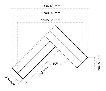
When laying the first row, make sure that the points and sides of the panels are perfectly aligned.
