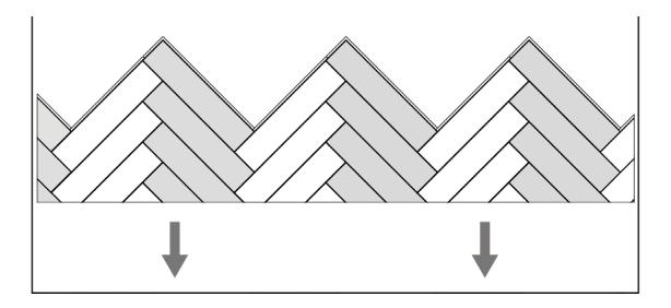
Push the sawn-off floor to 10 mm from the wall. Place spacer blocks between the wall and the floor. Continue finishing the floor.
