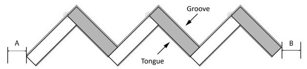
NOTE: Lay the first row in the center on the room and make sure that the points of the panels are perfectly aligned.
