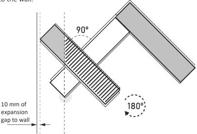
Rotate the right-hand board 180°, mark and neathly saw off at a 45° angle. Rotate the sawnoff piece 180° and click into the first floorboard. Do the same on the other side.
