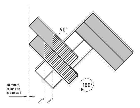
Further finishing is identical to the laying pattern for single herringbone, but with two floorboards.
