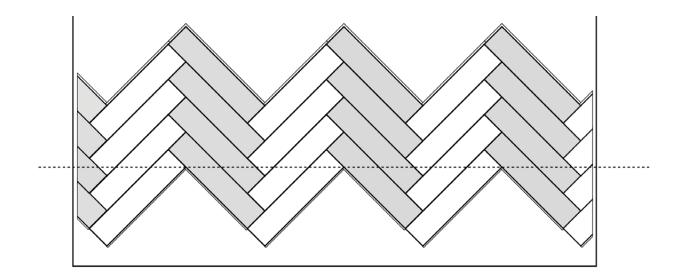
Continue to construct the floor row by row. Lay the left-hand boards first, and then the right-hand boards, on an alternating basis. Also finish the sides row by row.
