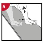
Press slightly along the short end just installed.
