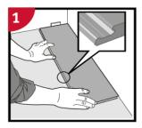
First floorboard, first row: Place a spacer of 15mm or %" thickness to the left and position the floorboard against the wall.
