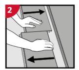
Your floor can very easily be dismantled, which enables replacement during and after installation. Separate the whole row by carefully lifting and slightly knocking just above the joint. Fold up and release the long side. Disassemble the floorboards by sliding horizontally. (Do not fold up, as this will damage the profile)
