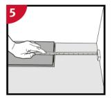
At the end of the first row, place a spacer of 15mm/ %" to the wall and measure the length of the last floorboard to fit.
