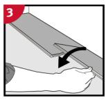
Fold the floorboard down in a single action movement.
