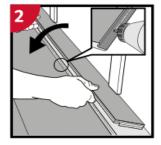
Cut the tongue at the same time you cut the length of the floorboard and install as shown above. Please note that the smallest width of a floorboard is 50mm/2" in the last row. If it is not, the first row width must be adjusted. This can easily be calculated when measuring the room width before installation.
