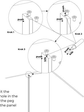
Click on the peg and fit the board into the fitting hole in the ceiling. Once in place, the peg will bounce and keep the panel inside.
